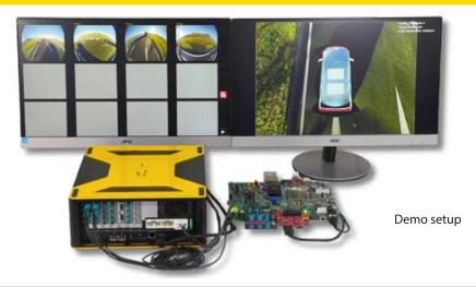
The logiRECORDER device injects 4 channels of video recorded by the test car's 4 video cameras furnished with integrated wide-angle (fish-eye) lenses, via a GMSL2 serial interface. The Surround View Parking Assistance ECU corrects the input video and stitches it together to provide a full 360° view.
